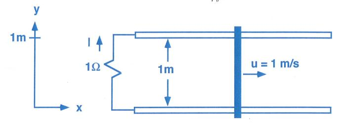
(10 pts)A) What is the current I, referenced as shown, flowing through the resistor is,
